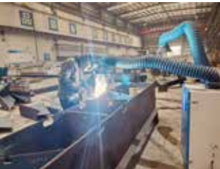
Mobile Welding Fume Collector
